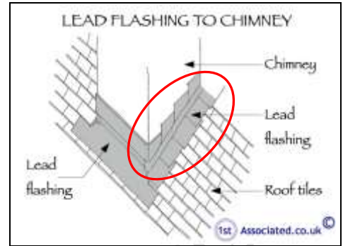
Example of step flashing highlighted in chimney sketch with red oval.
