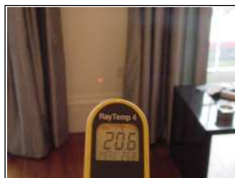
Five degrees warmer at the top of the room than the bottom of the room
