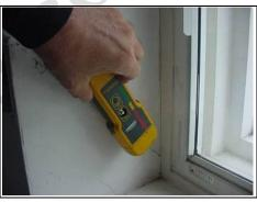
Testing for lateral dampness on the window reveals
