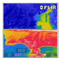
Thermal image showing heat loss out of a thatched roof
