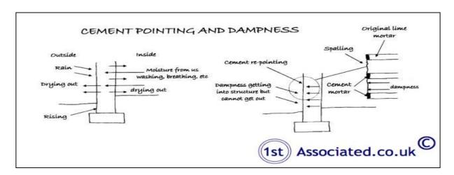
Use lime mortar every time instead of cement mortar to allow the property to breathe
