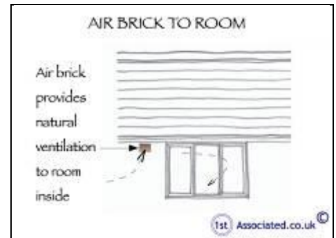
Air brick may not ventilate room enough
