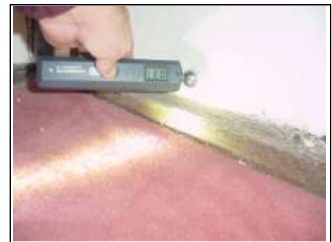
Testing for rising damp
