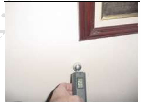
Testing for lateral dampness
