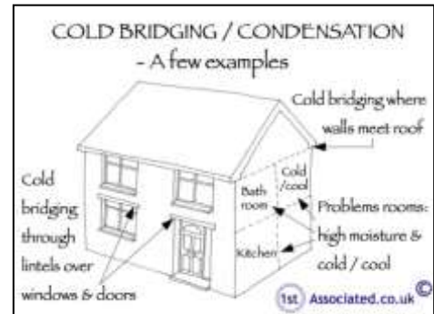
Cold bridging/thermal bridging
