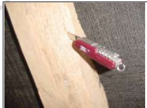
Woodworm with our knife going into the timber over an inch in depth
