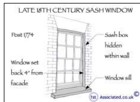
Later Georgian sash window
