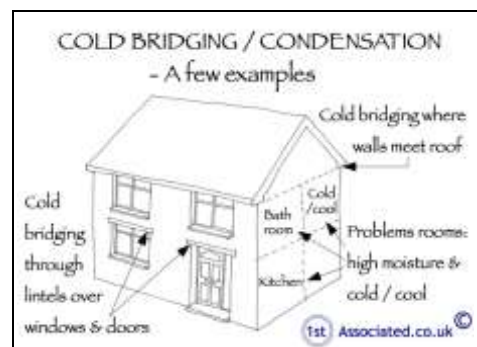
Thermal and cold bridging
