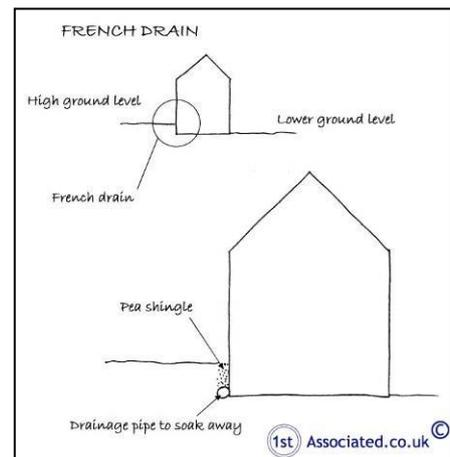
The French drain acts as an area where water soaks away quickly. We often recommend them close to building, but not next to the building, as this helps reduce the ground level and/or take any water that is directed at that area away. For example, where a patio has been put in place which aims any rainwater at part of the wall. As mentioned, whilst a French drain is a D.I.Y. job, it does need some understanding of how it works.
