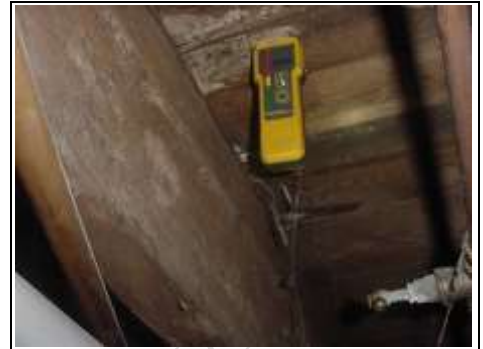
Dampness coming in through the flat roof
