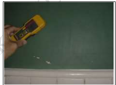
Lateral dampness coming through the walls
