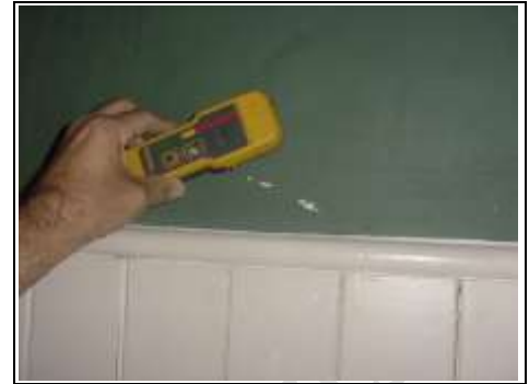
Testing for and finding lateral dampness!
