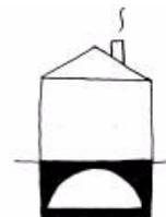
*Basements and vaults tend to be found in older properties and offer a useful space, although usually they are damp, unless some treatment has taken place such as the tanking of the walls, which is a lining process, or an external damp proofing membrane of some type has been added, or if internally the walls have been lined, therefore hiding the damp. Basements are often susceptible to flooding from excessive rain, rising water table levels or even blocked drains.*
